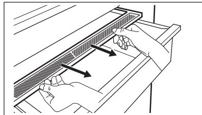
2. If you need to replace the device's white membrane, grab the device in the middle and separate the membrane from the cover by pulling the cover.
