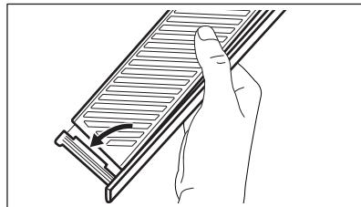
4. Reassemble the humidity control back on the drawer.
