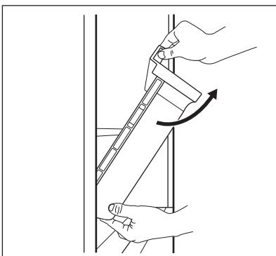
3. Lift and turn the drawer to pull it out of the appliance.
