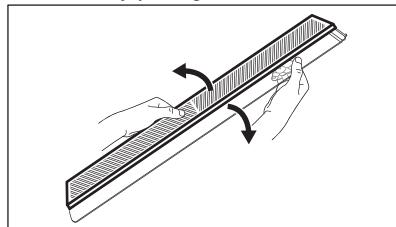
3. Assemble a new membrane into the cover by pressing the edge of the membrane into the cover.
