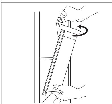
The shelf above the drawer can be removed from the appliance only for cleaning purpose.
