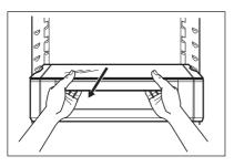
**2.** Tilt the module downwards to remove it from the refrigerator.
