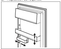
This model is equipped with a variable storage box which can be moved sideways.
