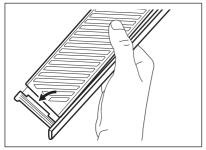
Reassemble the humidity control back on the drawer.
