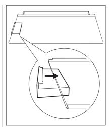
Insert the glass shelf back in the fridge compartment. Be careful not to hit the filter when inserting the glass shelf.
