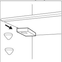
Replacing the air filter
