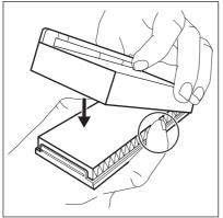
Remove the top glass shelf from the fridge compartment. Slip the plastic housing with the air filter on the left side of the glass shelf.
