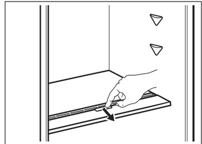
To remove the humidity control device, open the drawer below the glass shelf and pull out the cover.
