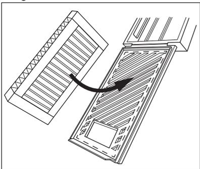
3. Hold the filter down while closing the plastic housing until you hear a click.
