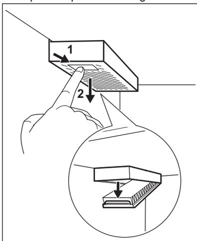
2. Pull out the used air filter.
