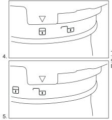
To Lock/Unlock the cartridge, refer to Picture 4 and 5:
