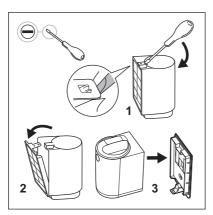
1. Remove the filter from packaging box and remove the wall support with the help of a flat screwdriver.
