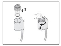
Before proceeding to the next topic Daily use & care and cleaning, start the short washing programme and follow it until the end. Be sure that no leakages appear from the filter and its connections. In case of water leakage, proceed as described in paragraph 8. Detach the filter assembly from the wall support and tighten the collars. To reinstall the filter, repeat the steps in paragraph 7.
