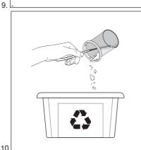
After the water has been emptied from the cartridge, remove any dirt and mircrofibres from inside the cartridge and dispose of it in DRY general waste. A paper towel can be used to collect as much material as possible.
