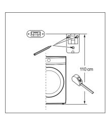
b. Use a level to check that the 3 drilling punches are level and well-aligned before drilling.
