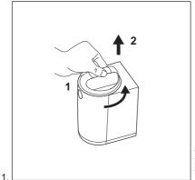
To open the filter, refer to the movements in Picture 1 and 2:
