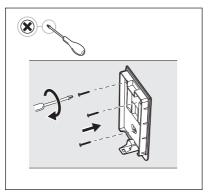
3. Drill the holes into the wall and place the anchors.
