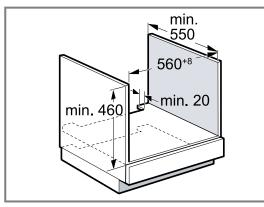
The worktop must be secured to the fitted unit.
