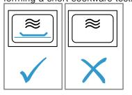
If you prepare microwave popcorn at a microwave power level that is too high, the door pane may crack due to overloading.
