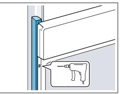
3. Secure the appliance using a suitable screw.
