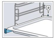
**Note:** Gently push the pull-out rails back into the cooking compartment.
