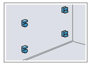
1. Hook the front retainers with the hook into the round hole at the top and set them at a slight angle  $\bigcirc$ .
