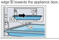
**3.** To place the accessory at shelf positions with pullout rails, pull out the pull-out rails.
